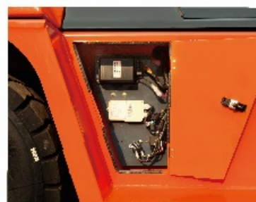
独立集成电控箱 Independent integrated electric cabinet
